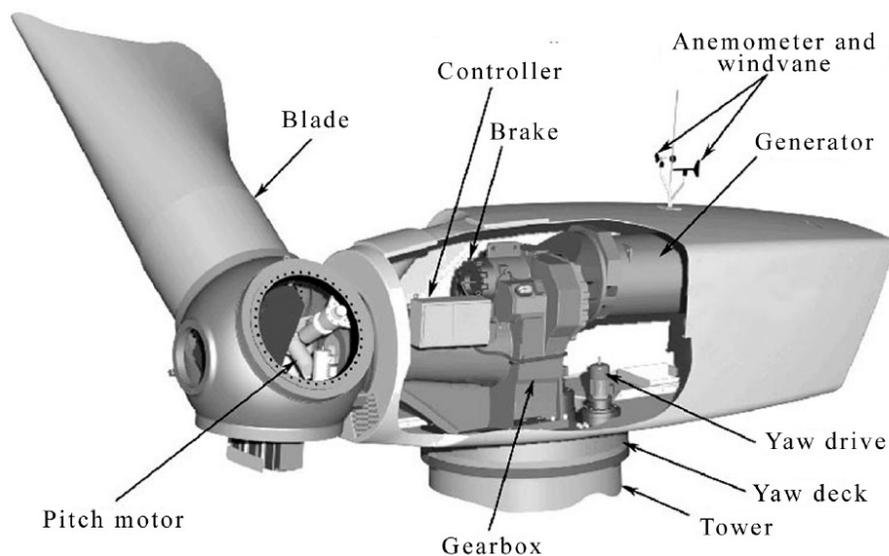
Figure 2-1 (Manwell et al) Annotated diagram of system components
