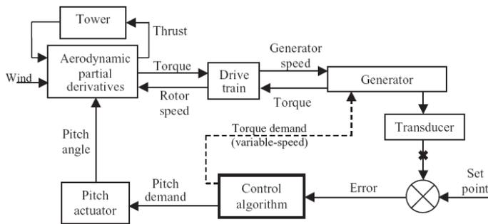
Figure 8.9 Typical Linearized Turbine Model
